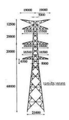
Fig. 3. Configuration of towers
